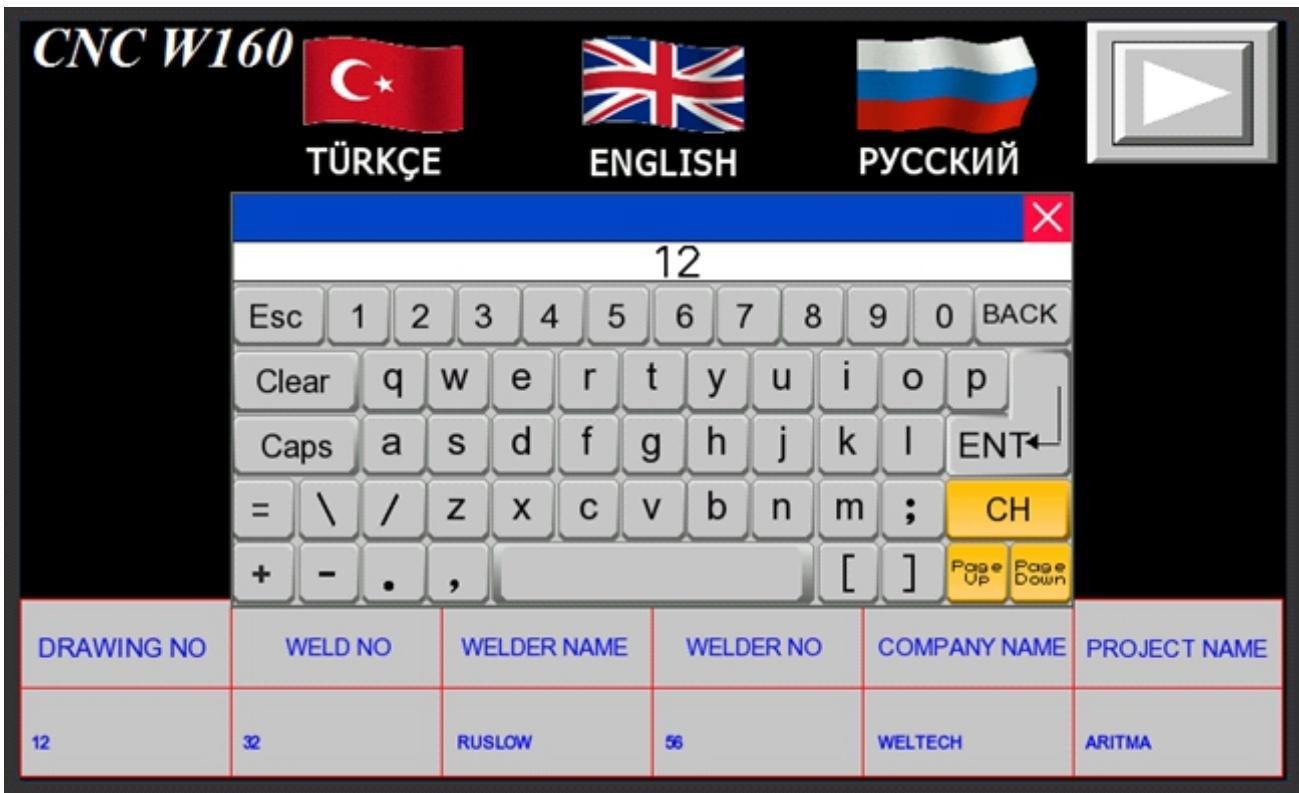
13-On the operator panel choose language by touching the flag and set pipe material, pipe diameter and PN class and fill company name, welder name and project name than touch to button and pass to next screen. Below the panel plug in a USB flash drive to getting welding results after welding operations.
