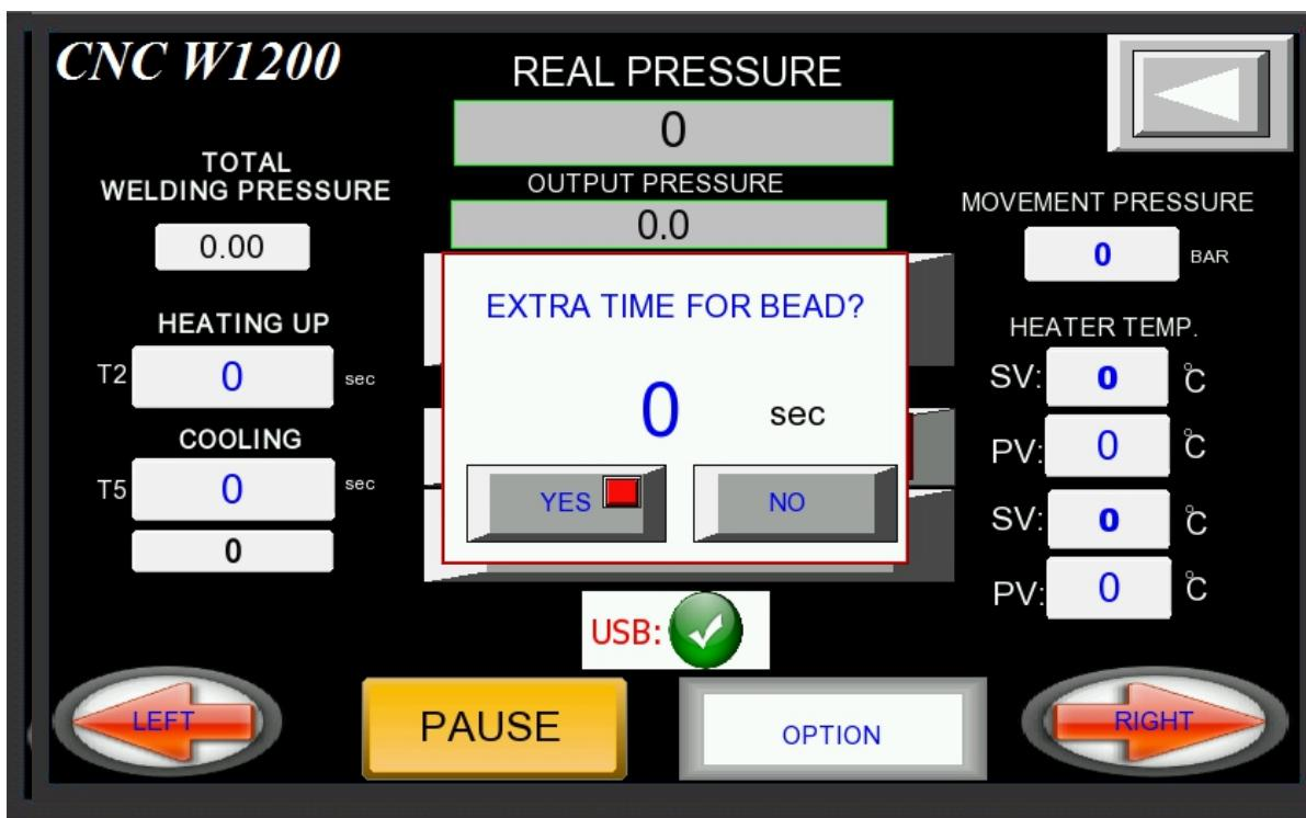
16-After setting the heater on the machine touch
