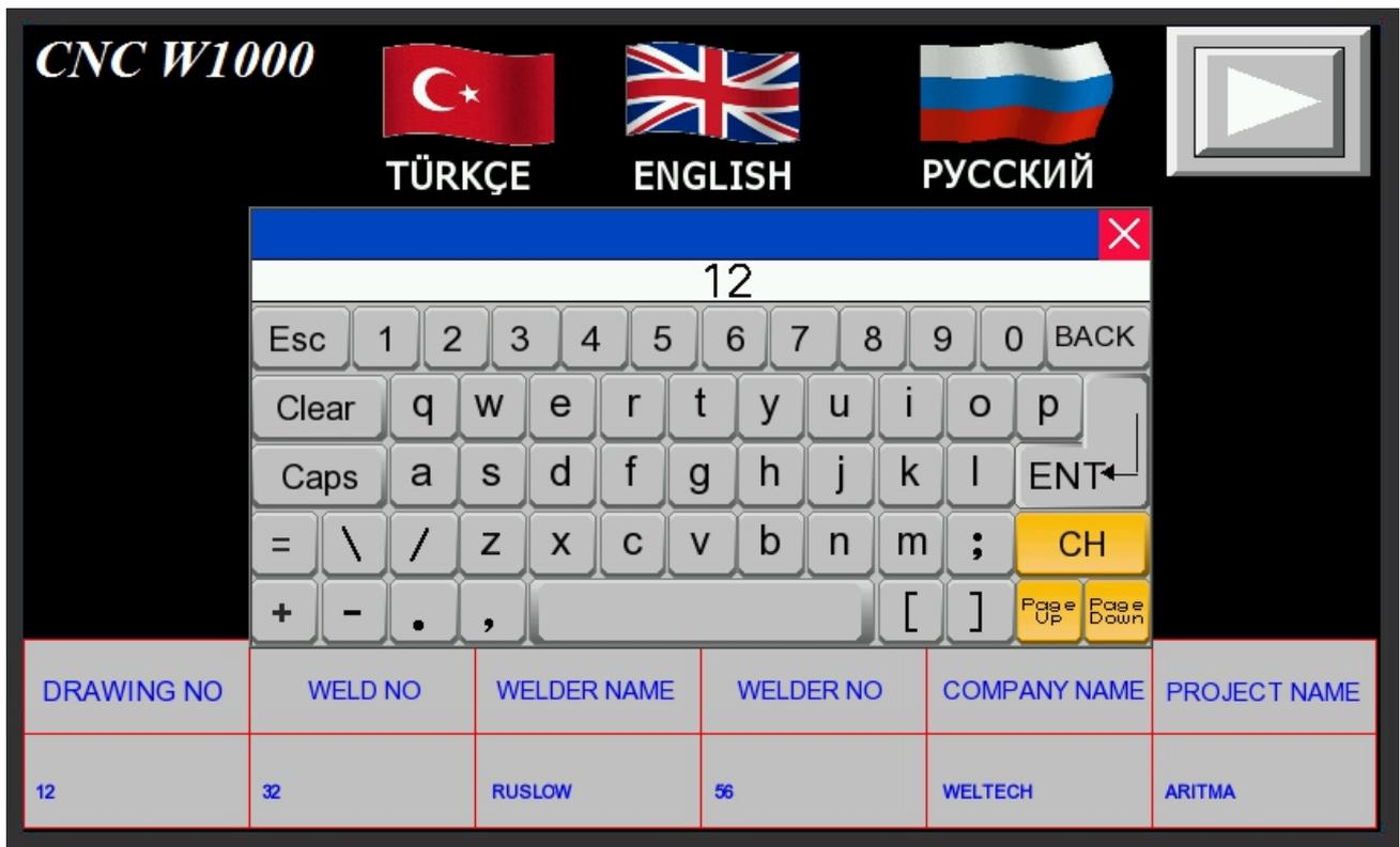
13-On the operator panel choose language by touching the flag and set pipe material, pipe diameter and PN class and fill company name, welder name and project name than touch to
